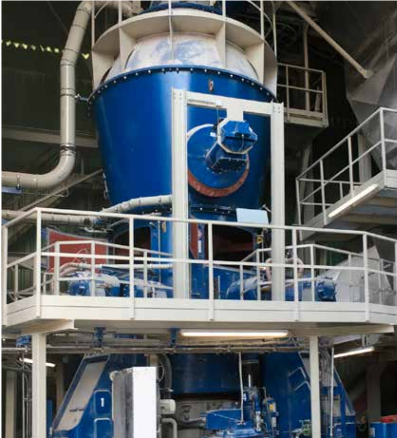
3 MVR 1800 R-4 with grit extraction for grinding of limestone
