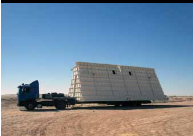
Figure 4: complete preassembled process filter bottom hopper
