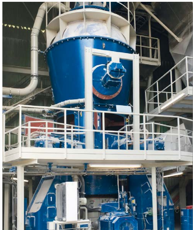
Figure 2: First MVR vertical roller mill for fine grinding of limestone – product fineness degrees up to 0.1 % R 20 µm
