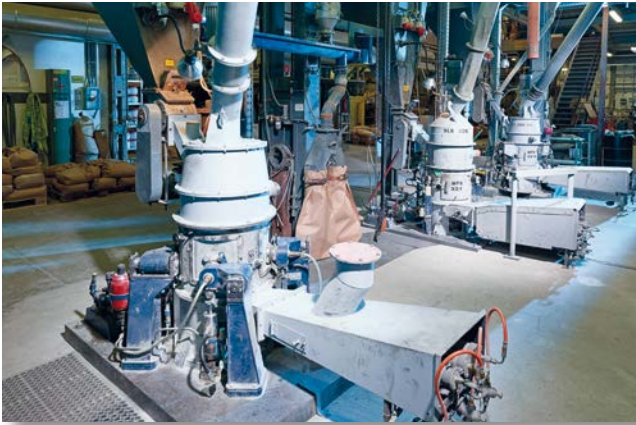
Figure 5: Gebr. Pfeiffer's test station – test mills – MVR 400 in the foreground, MPS 32 in the background
