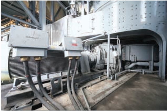
Figure 3: MultiDrive® with three 1 450 kW drive modules in the Val de Seine grinding plant in France
