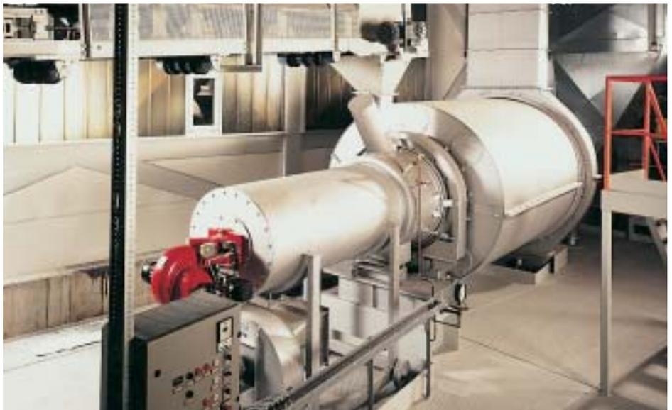
Triplex dryer with hot gas generator
