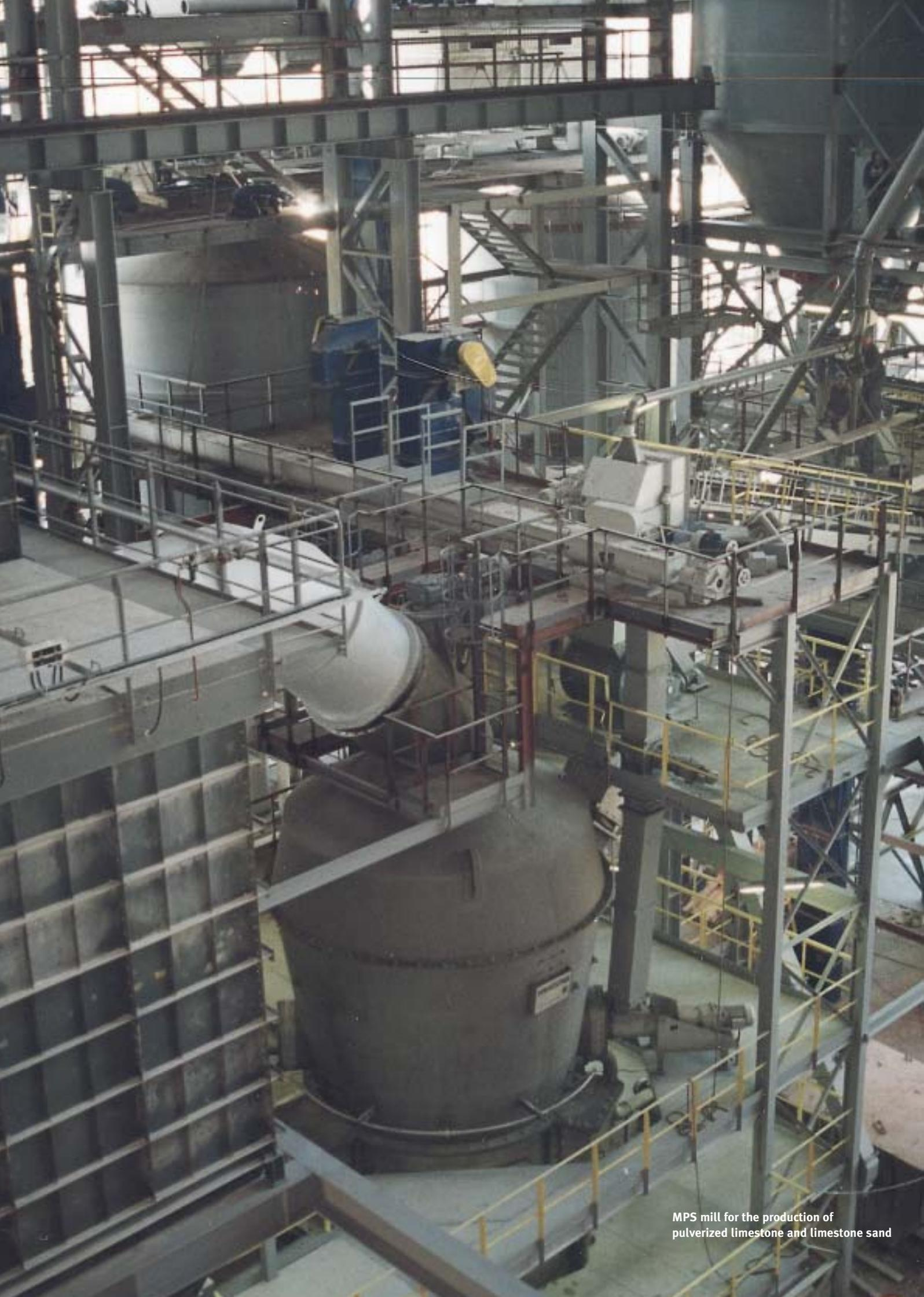
MPS mill for the production of pulverized limestone and limestone sand
