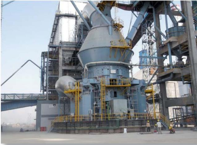
Figure 2: View of the Gebr. Pfeiffer mill MVR 6000 C-6 at the Raipur plant
